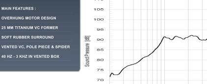
The C153 - 4 - 082 is a 5 inch bass - midrange driver with ultra hard ceramic dome.
