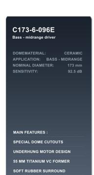
The C173 – 6 – 096E is a 6.5 inch bass-midrange driver with ultra hard ceramic dome.
