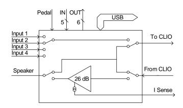
Internal connections for impedance measurements (Internal Mode)
