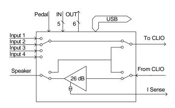
Internal connections for frequency response measurements
