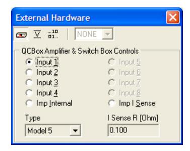
Choose Model 5 in the 'Type' drop down. The control should be active; an acoustic confirmation should come from the internal relays, you should hear them clicking when changing inputs.
