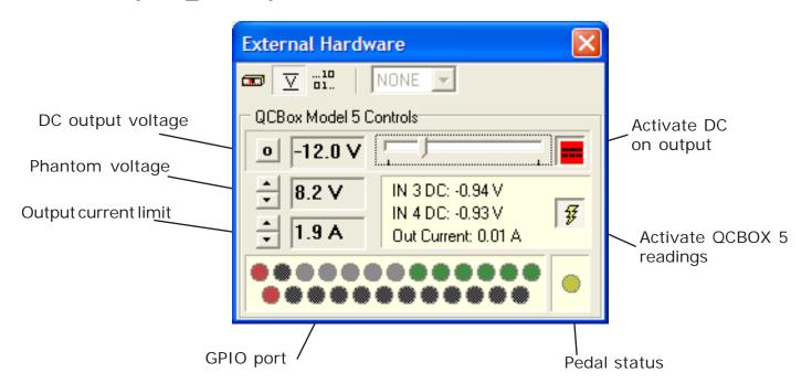
Using this panel is possible to choose the DC output voltage, the phantom voltage, the output current limiter. The GPIO port can be wrote simply by clicking on the output bits.
