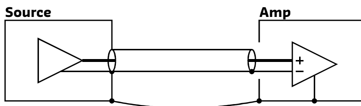
Figure 1: The basic idea behind a differential (floating) input.
