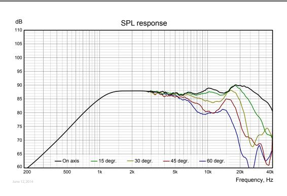
Measuring conditions, SPL Driver mounting: Flush in infinite baffle, back side open (no cabinet) Microphone distance: 1.0 m Input signal: 2.83 VRMS stepped sine wave Smoothing: 1/6 oct.
